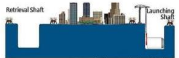
2. Assemble the TBM at the launching shaft
