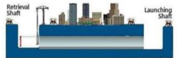
4. TBM arrives in the retrieval shaft to be dismantled for transportation
