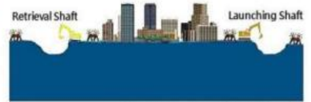
1. Excavate launching shaft and retrieval shaft
